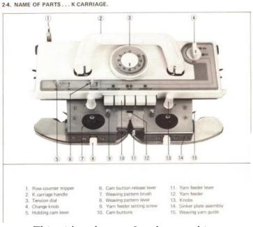
Left: shows the carriage, with the holding cam lever on the left side. This needs to be set to H.
