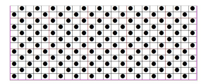
● – Hole in Punchcard or Needle selected to upper working position for tuck stitch.
