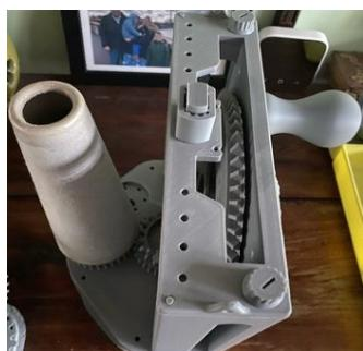
3d printed hand wound cone winder: a complex print, but works reasonably well: [Cone winder for CSM by Yarnico](#) | Download free STL model | [Printables.com](#)
