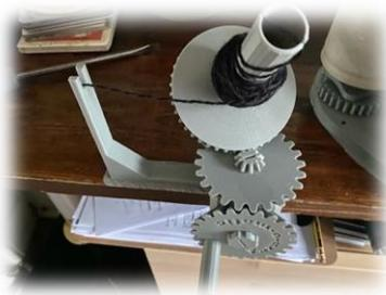
3d printed yarn winder - economical use of filament, useful for small amounts of yarn. [estimated cost around £2-3]
